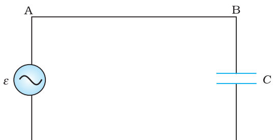
FIGURE 7.7 An ac source connected to a capacitor.
